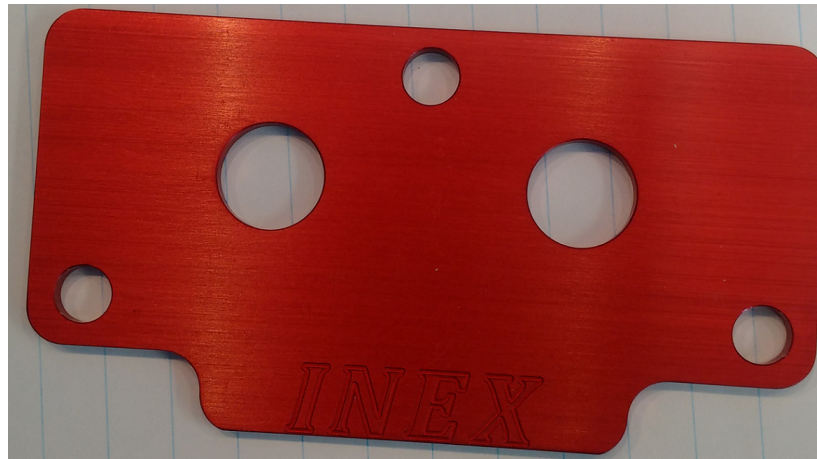
\frac{1}{2} inch opening red restrictor plate
